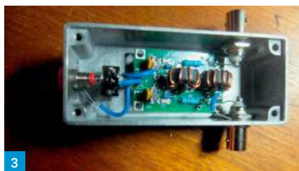
Fig. 1: SWR bridge circuit.
